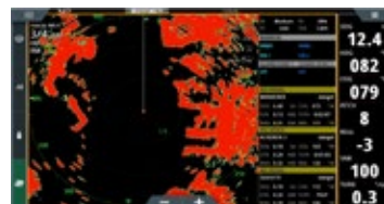
A faster rotation speed allows a faster refresh of targets in the PPI (radar screen).
