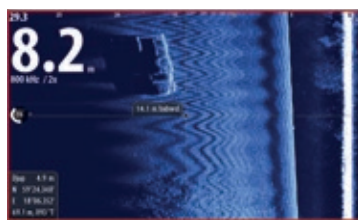
Underwater truck wreck (showing the left hand side of a SideScan view)
