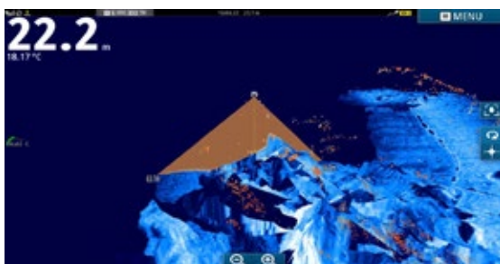
StructureScan® 3D showing fish-holding around rocky structure near Nelson, New Zealand. Use Vertical Enhancement to make smaller structure appear larger and more visible.
